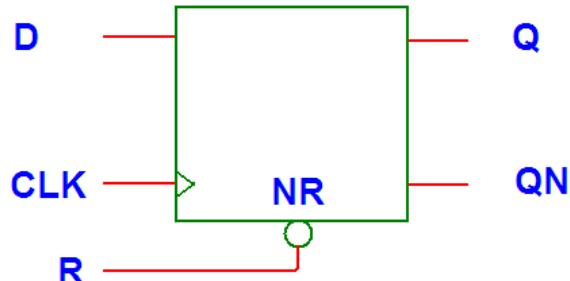
In **D**-Type of flip-flop whatever input is applied to **D** will be transferred to the **Q** output as soon as the clock goes high, provided that the reset is not active, (*i.e reset is low = 0*). The **Q** output will be immediately reset to **0** irrespective of the low or high data in **D**-input if reset is active (*i.e reset is high = 1*). The truth table for **D**-Type of flip-flop is given below.
